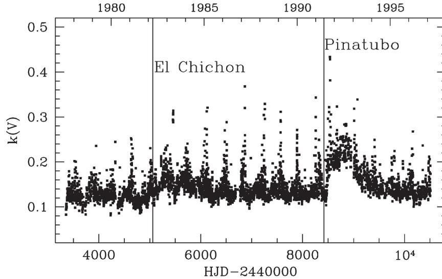
Figure 2. Variations of the extinction coefficient in the  $V$  band during photometric nights at La Silla Observatory. The effects of the stratospheric aerosols (sulfur dioxide transformed into sulfuric acid) from the two volcanoes El Chichon (Mexico) and Pinatubo (Philippines), and of meteorological aerosols (global annual variation due to the haze and dust content of the atmosphere above the site) are clearly visible (for more details, see Burki *et al.* 1995).
