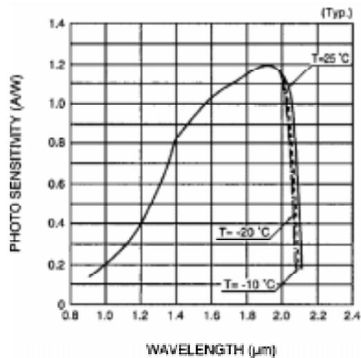
Figure 2. Spectral response curve for the Hamamatsu G5852 InGaAs PIN photodiode. Courtesy Hamamatsu Corporation.
