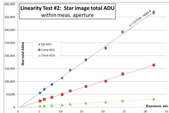
**Figure 5: Linearity test (integrated ADU vs exposure duration).**
