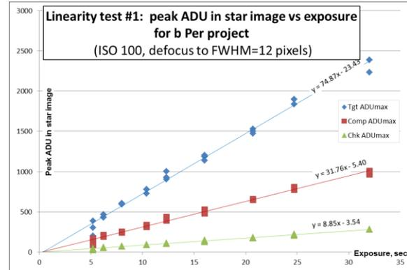
**Figure 4: Linearity test (peak ADU vs. exposure duration).**
