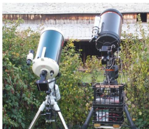
**Figure 2.** Grand View Observatory telescopes configured for simultaneous photometric and spectrographic observing runs. The wider aperture of the Celestron 14-inch permits 9th magnitude star spectra to be acquired in the same time that the Vixen 10-inch can acquire a set of BV, VR, or RI photometric data, about 20 minutes.
