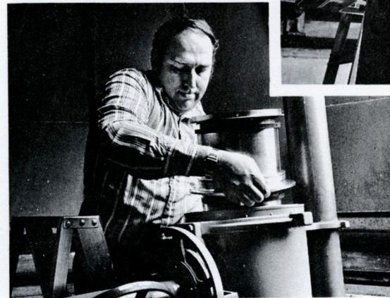
*Paul Valleli of Optical Sciences and Technology, Inc. returning the Cooke lens to the photographic telescope after adjusting it.*
