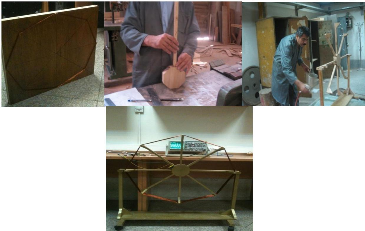
Figure 3 Different phases of building the octagon antenna:
