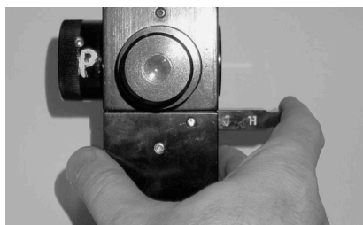
Move slider in: squeeze between thumb and forefinger
