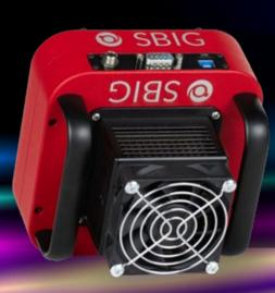
The ALUMA AC2020BSI uses the Gpixel GSENSE2020BSI™ CMOS sensor with 4 million pixels at 6.5 microns in a 2048 x 2048 array. The sensor measures just over 13.3 mm square. Similar in detector size but lower in cost than the ALUMA CCD47-10.
